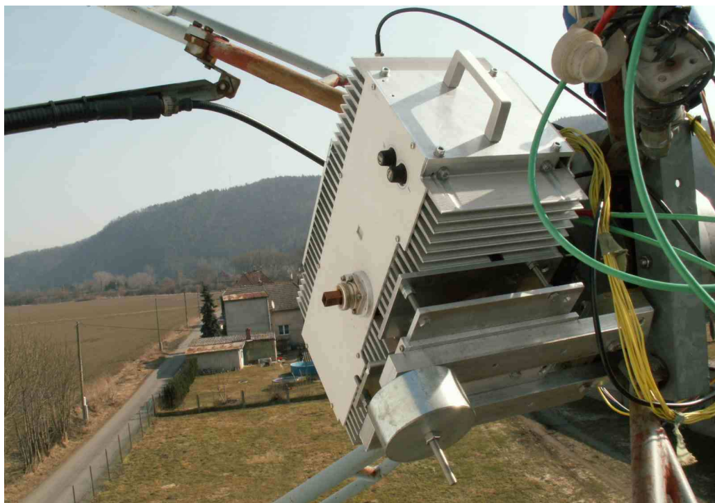
OK1KIR is back on 24GHz EME after 3 years break. Completely redesigned 24 GHz TRX (SSPA) weights itself over 16kg, produces \approx 23\text{W} at the feed, \text{NF} \approx 1.5\text{dB} . TRX box is placed on remotely controlled rotatable 'L shape' holder in the focus of 4.5m dish. Heavy cylinder at the bottom balances the gravity centre to the axis of rotation.
